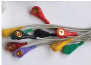
Picture 4a. ECG leads – European colors and labels
