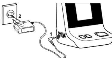
To disconnect the power outlet, unplug the AC adapter from the power outlet first and then remove the AC adapter plug from the unit.
