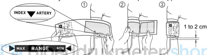
Make sure that the INDEX ARTERY "▼" is within the range. If outside the ►MAX RANGE MIN◄ range, there will be greater error in the blood pressure value. In this case, use the appropriate cuff size.
