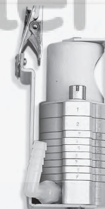
Cascade Impactor Mechanical impact-based particle sizing method
